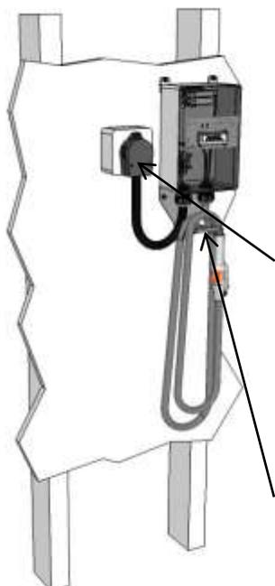
The **TucsonEV-SE** is supplied with 4 lag bolts for stud mounting. Suitable fasteners may be needed for mounting in other types of materials such as concrete blocks.
