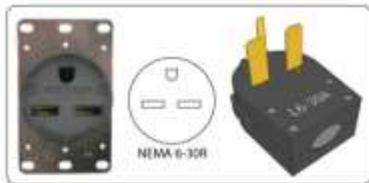
A NEMA 6-30Amp /50Amp plug is supplied which can be configured as either a 30 Amp plug or a 50 Amp plug. It comes configured as a 50A plug. The **TucsonEV-SE** power plug should be plugged into a dedicated 6-50 Amp receptacle or a dedicated 6-30 Amp receptacle. The **TucsonEV-SE** has the 50A version configured and if you chose, you can change the plug to the 30A version with the included 30A leg.
